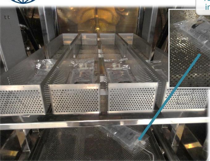
Temperature probe inside the sample
