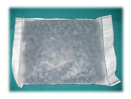
A typical example of a porous solid load to be treated in a saturated steam autoclave
